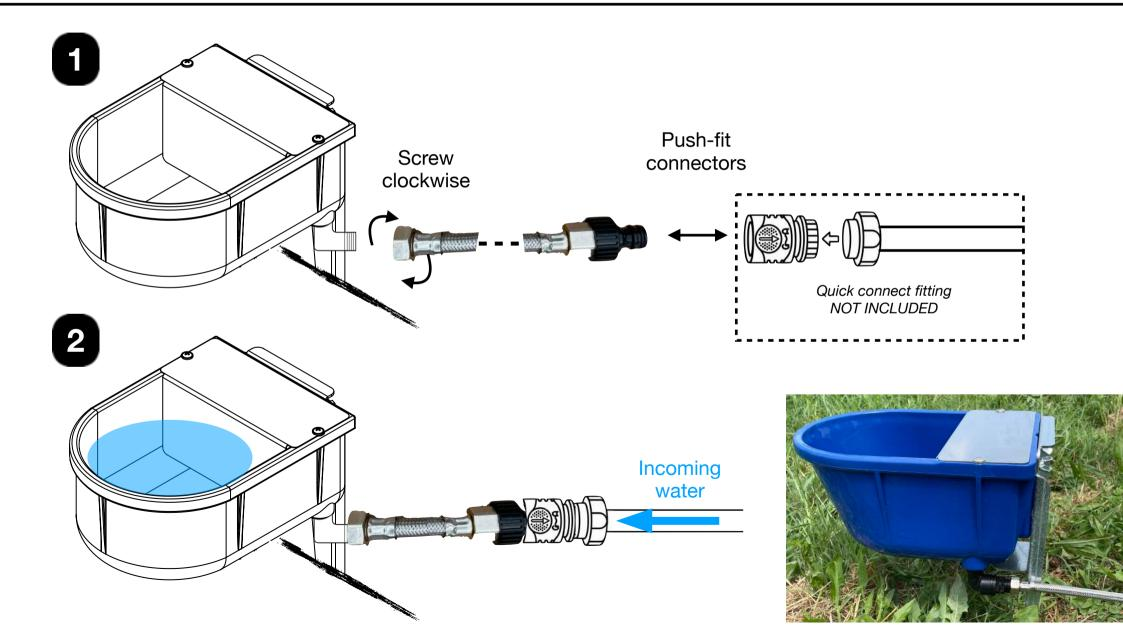
To ensure the best performance and maximum life of our equipment, we recommend using only original spare parts. Do not hesitate to contact us: we will be happy to provide you with what you need. It is also recommended not to replace the fittings without first consulting the company: using a fitting with an unsuitable thread can compromise the correct functioning of the drinker and cause damage.
